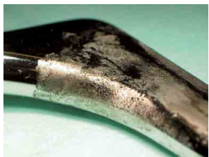
Implant corrosion observed on the stem of an explanted component.
